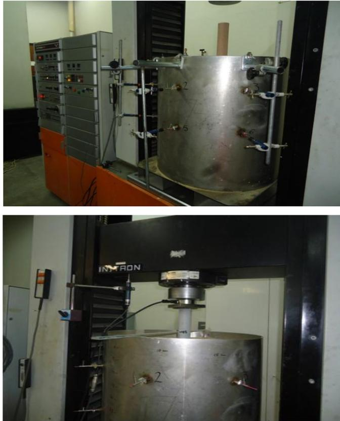
Figure 2: Pile inside the Sand Box for Testing
